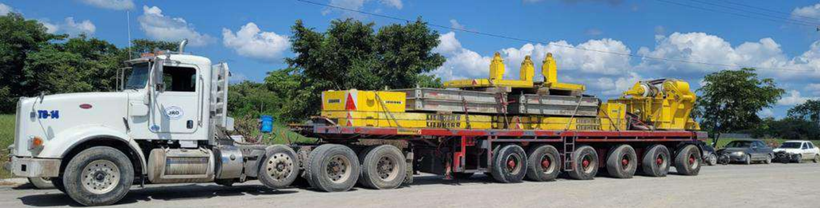
Modular Platform 48 ft Capacity: 75 tons
